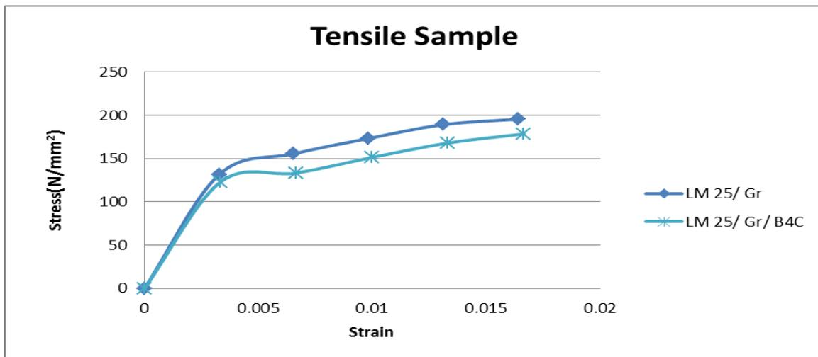
Figure 3 Stress vs strain curve of LM 25/Gr and LM 25/Gr/ B<sub>4</sub>C MMC's
