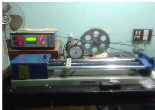
Figure 2 Micro Tensile Test - Digital tensometer
