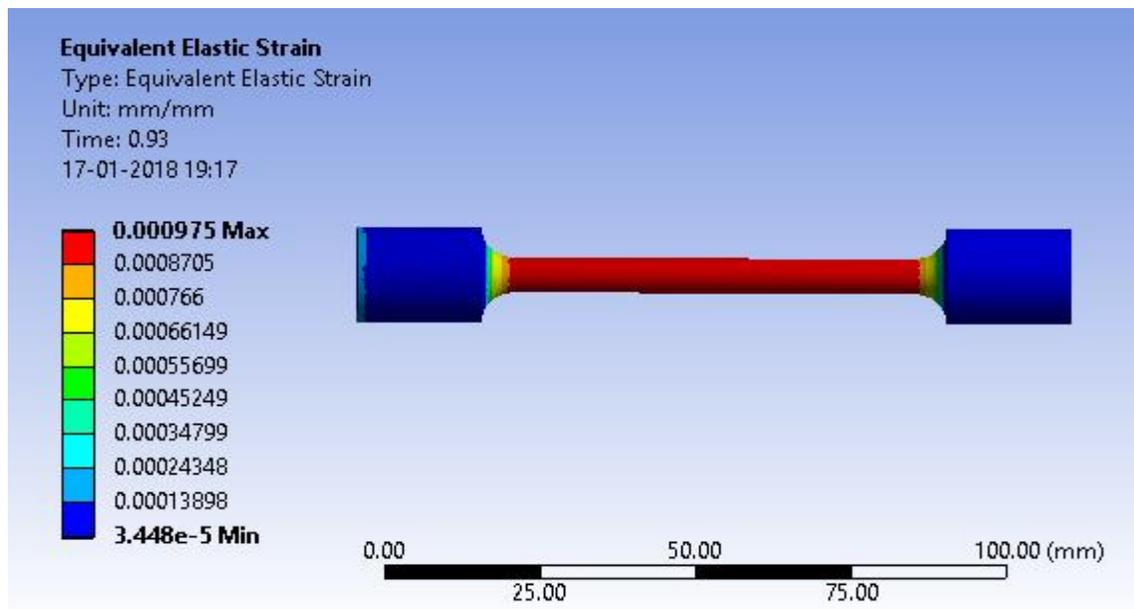
Figure 6 Equivalent Strain Plot
