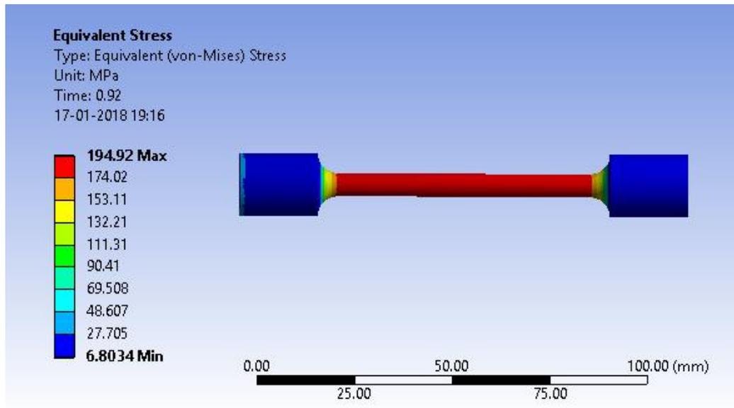
Figure 5 Equivalent Stress Plot
