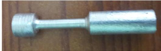
Figure 1 Tensile test specimen
