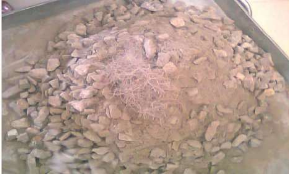
Figure: Materials required for Rigid Pavements
