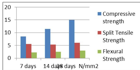
**Fig 5 Flow Chart for Partially Replacing of Plastic Coarse Aggregate with Concrete Compression Strength, Flexural Strength and Split Tensile Strength Results for M25 Grade of Concrete**
