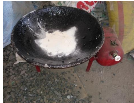
Fig 2: Bitumen Mix With Egg Powder
