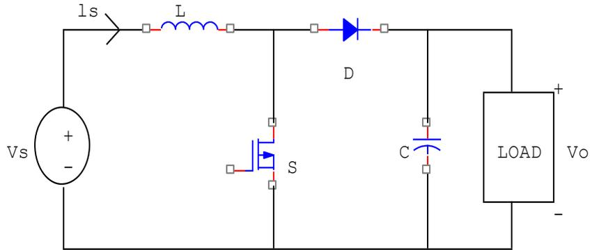
**Fig 2: DC-DC converter circuit**
