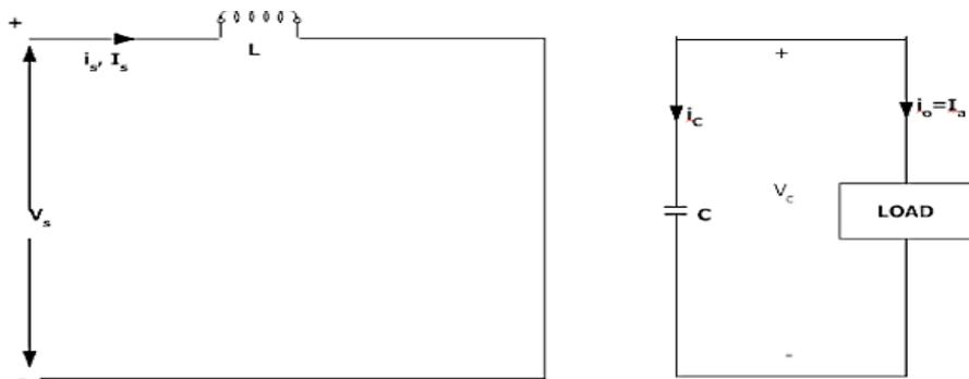
**Fig 3: Circuit operation Mode1for boost converter**
