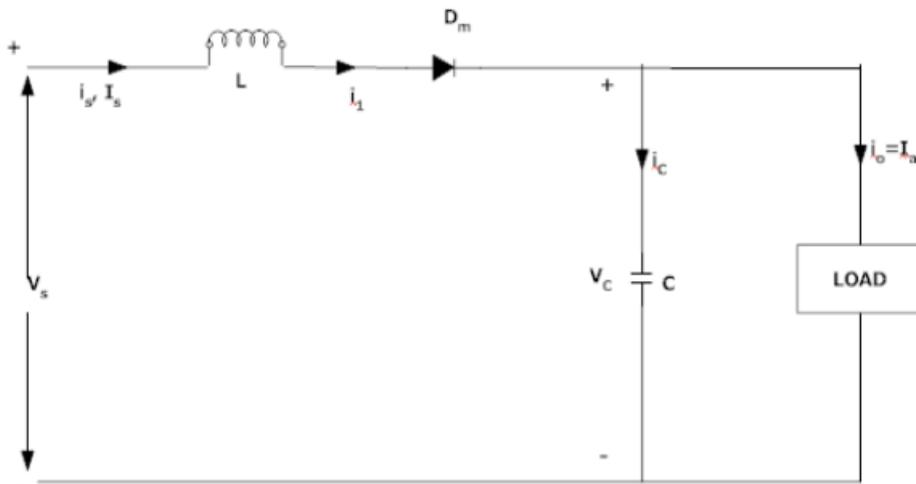
**Fig 4: Circuit operation Mode2 for boost converter**
