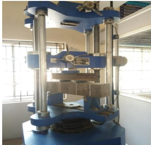
Fig 3: Flexural strength testing of prism
