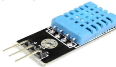
**Fig 4: Humidity sensor (DHT11)**
