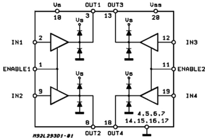
Fig 1: Motor driver Circuit
