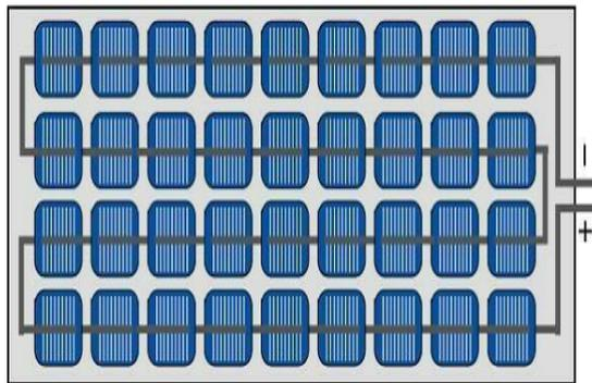
**Fig 2: Structure of a PV module with 36 cells in series**
