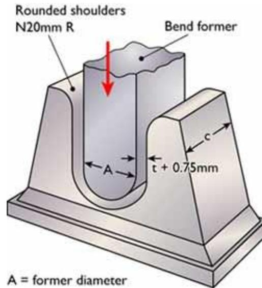
Fig. 7 shows a driven bend test jig with a male and female former, which is the most common type of equipment
