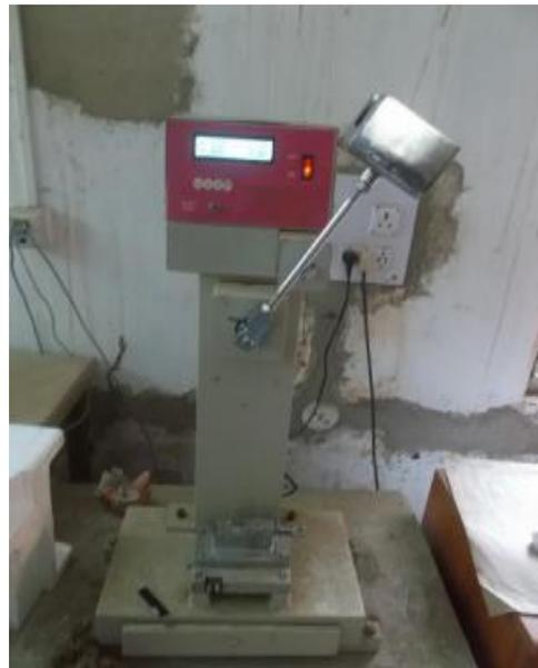
**Fig. 4 Experimental set up for Impact strength test**
