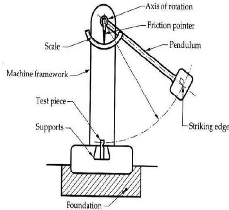
**Fig. 5 Izod Test equipment**
