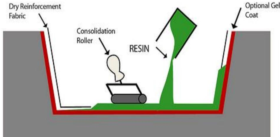
**Fig. 2 Hand Lay-up Technique**
