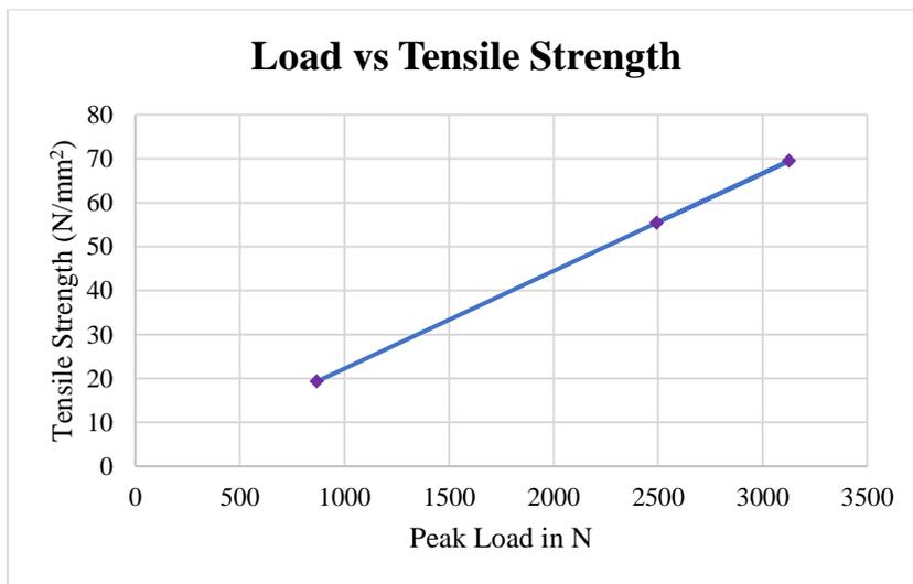
Fig. 12 Load vs Tensile Strength
