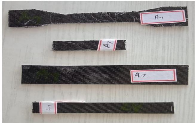
**Fig. 10 A7 – Carbon Fibre + Jute Fibre**
