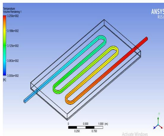
**Fig. 7 Temperature Difference air flow rate in 0.01kg/s at 60min (Square)**
