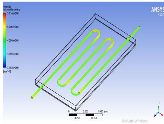
**Fig. 6 Velocity difference in Circular Tube**
