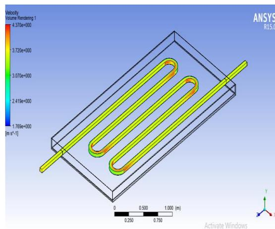
**Fig. 9 Velocity difference in Square Tube**
