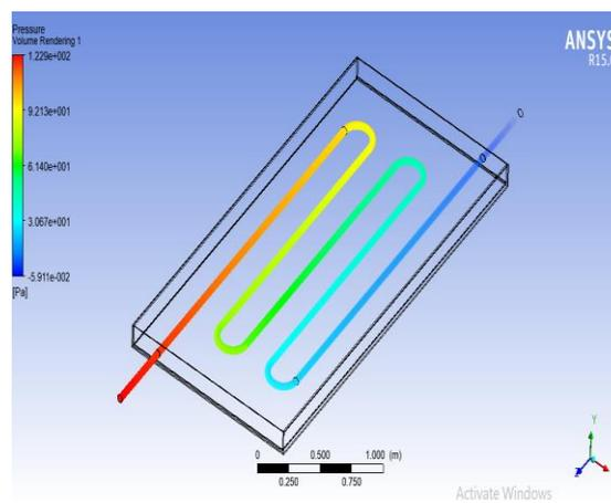
**Fig. 5 Pressure difference in Circular Tube**
