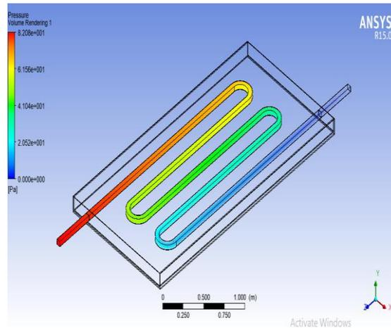
**Fig. 8 Pressure difference in Square Tube**
