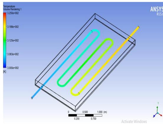
**Fig. 4 Temperature Difference air flow rate in 0.01kg/s at 60min (Circular)**
