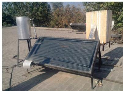
Fig. 1 Flat Plate Collector
