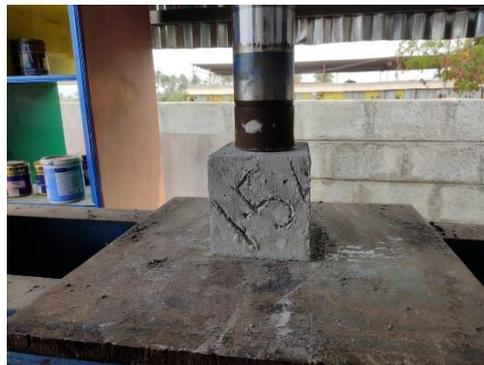
**Fig 4.1 Compression Test**
