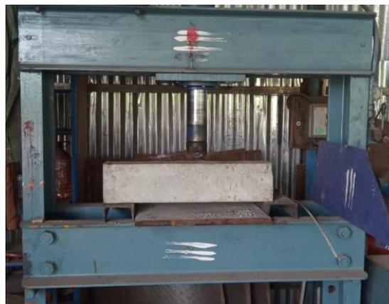
**Fig 4.3 Flexural Strength Test**
