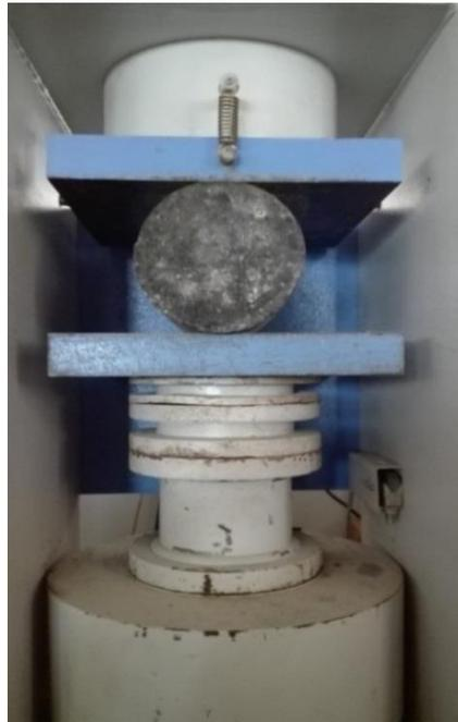
**Fig 7.2 Split Tensile Strength Testing of Cylindrical Specimen**
