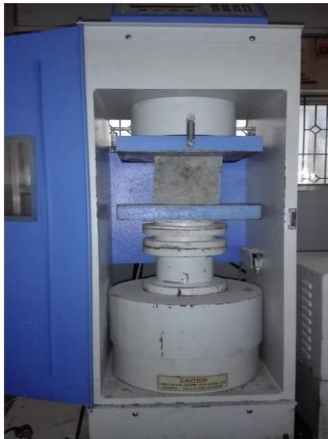
**Fig 7.1 Compressive strength testing of cube Specimen**
