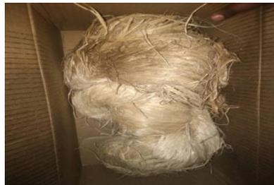
**Figure: 3.2 banana tree fibre**
