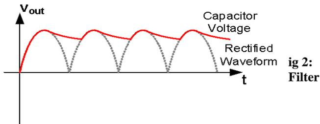
If a Capacitor is added in parallel with the load resistor of a Rectifier to form a simple Filter Circuit, the output of the Rectifier will be transformed into a more stable DC Voltage. At first, the capacitor is charged to the peak value of the rectified Waveform. Beyond the peak, the capacitor is discharged through the load resistor until the time at which the rectified voltage exceeds the capacitor voltage. Then the capacitor is charged again and the process repeats itself shown in fig2.
