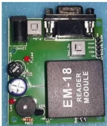
FIG-6 Hardware Rfid Reader
