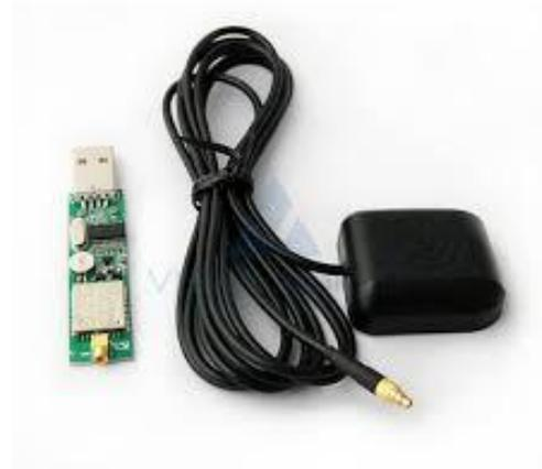
Fig. 3. SIM300 and EB-3531 with external antenna
