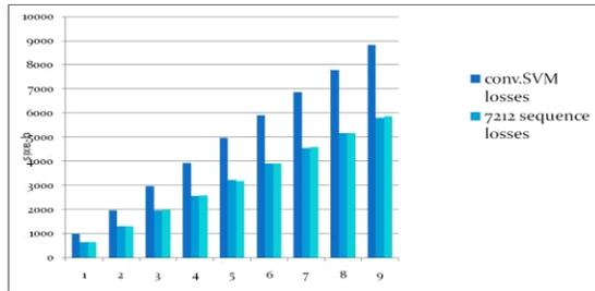
Fig. 10 Comparison of switching losses with conv.SVM ,0121 and 7212
