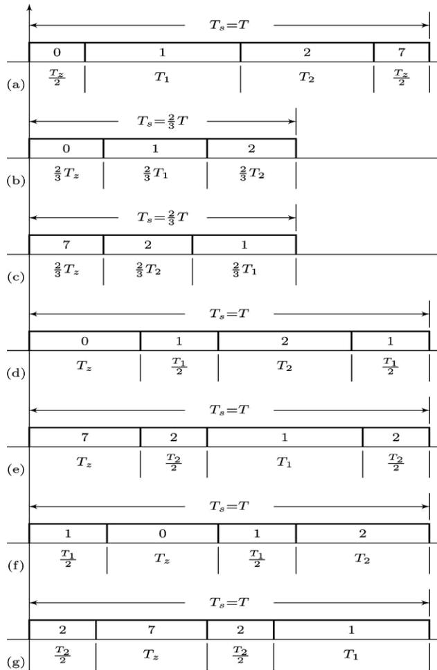
Fig. 4 Seven possible switching sequences in sector I: (a) 0127, (b) 012, (c) 721, (d) 0121, (e) 7212, (f) 1012, and (g) 2721.
