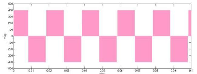
Fig 13. Lower line to line output voltage with the lower Modulation index ma=0.82 and measured voltage is V lower(rms) =310 volts
