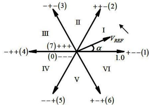
Fig .3 Voltage vectors of a VSI. Magnitudes of the vectors are normalized with respect to dc bus voltage  $V_{dc}$ . I–VI are sectors.
