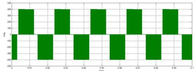
Fig 12.Upper line to line output voltage with the upper Modulation index ma=0.9 and measured voltage is V upper(rms) =370 volts
