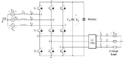
Fig 11. Hybrid topology for nine switch rectifier-inverter topology
