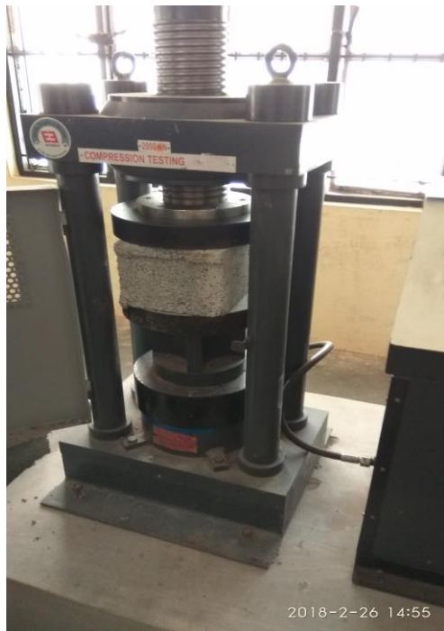
Fig.3 Compressive strength test
