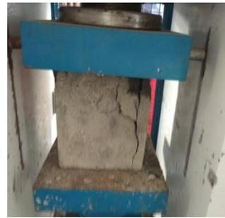
**Fig 4.1 Compressive strength test**
