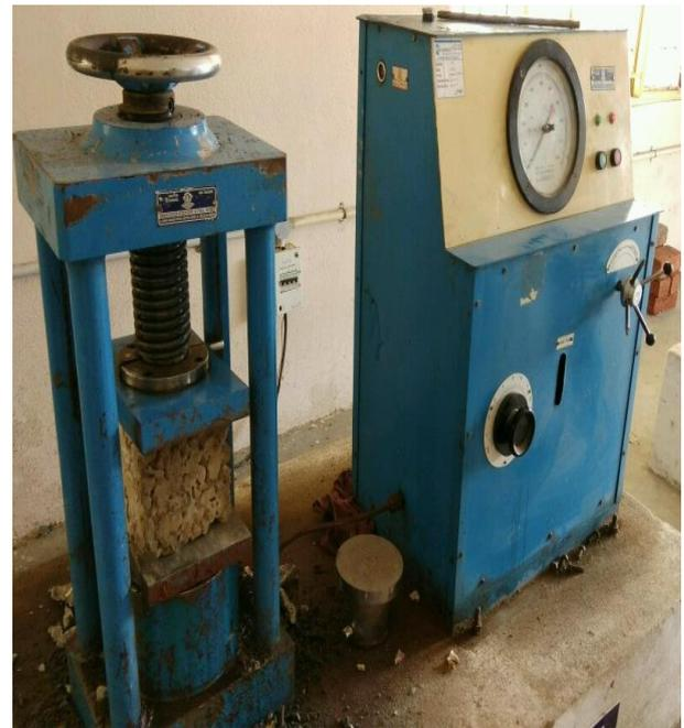
**Figure No 1: Compressive test on prism**
