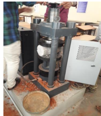
Fig No 6: Testing of cylinder
