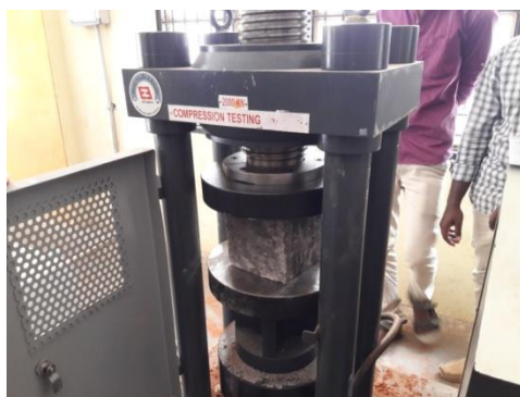
Fig No 3: Testing of cube
