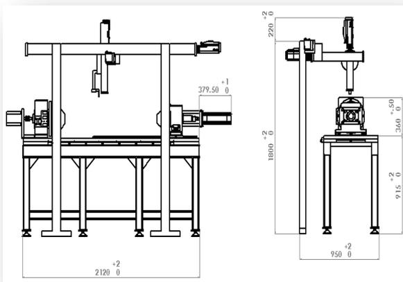
Fig. 4 Machine Layout
