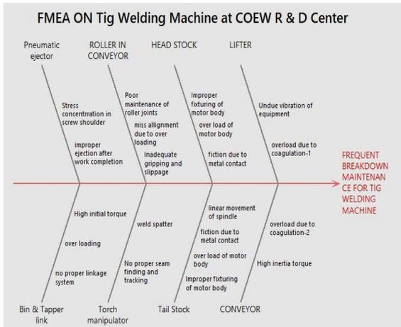
Fig. 5 Cause and Effect Diagram
