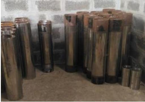
Fig. 2 Manually Welded pump motor body
