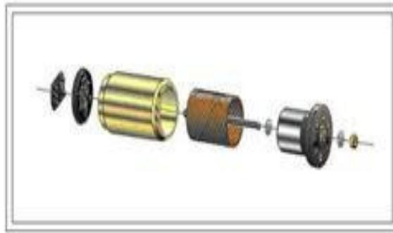
The use of an iron core armature (as in the Mabuchi, above) is quite common, and has a number of advantages. First off, the iron core provides a strong, rigid support for the
