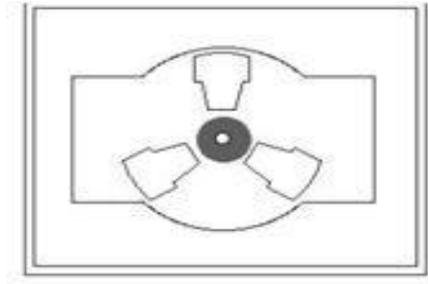
A few things from this -- namely, one pole is fully energized at a time (but two others are "partially" energized). As each brush transitions from one commutator contact to the next, one coil's field will rapidly collapse, as the next coil's field will rapidly
