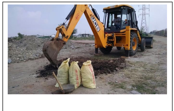
of Village Road by 2025, as Village Road usually demands sub base strengthening at a cheaper cost. Given the scale of Fig 2 Soil specimen collection
