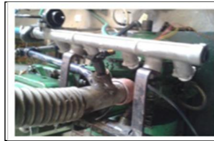
Fig 2. Common rail fitted in intake pipe
