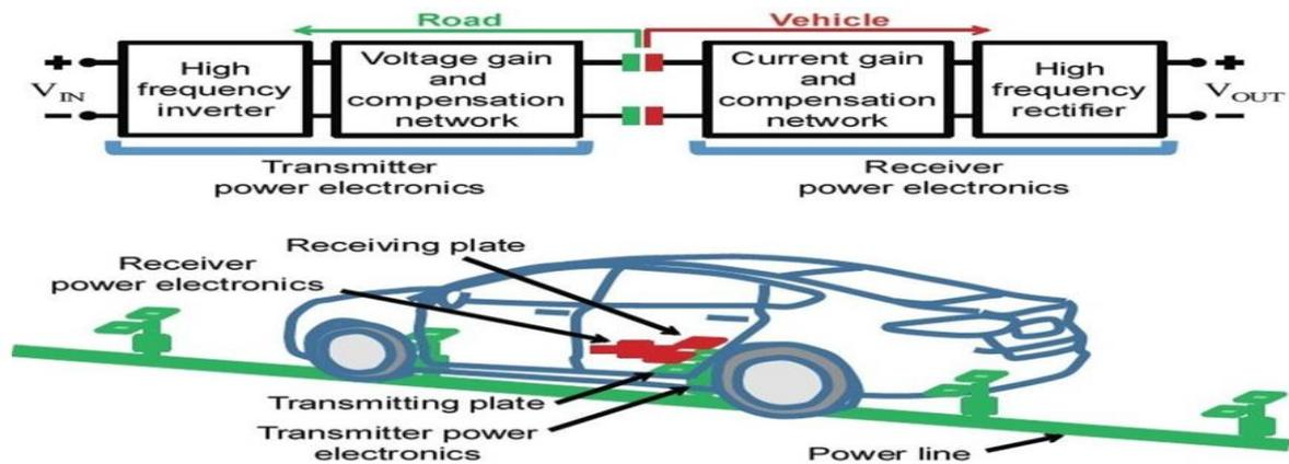
Figure1 power transfer using plates
