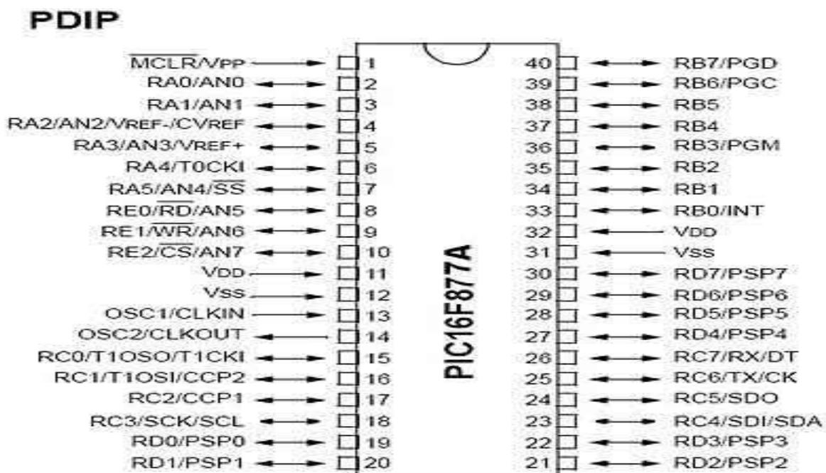
Figure 1: Pin configuration of PIC16F877A
