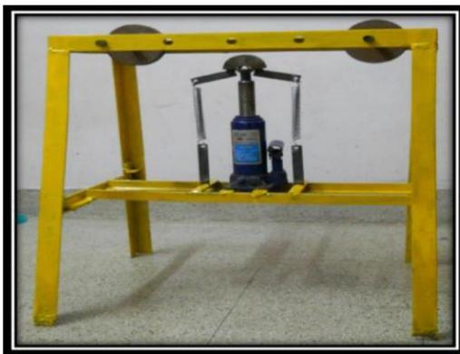
Fig. 1. Design details of Hydraulic Pipe Bending Machine
