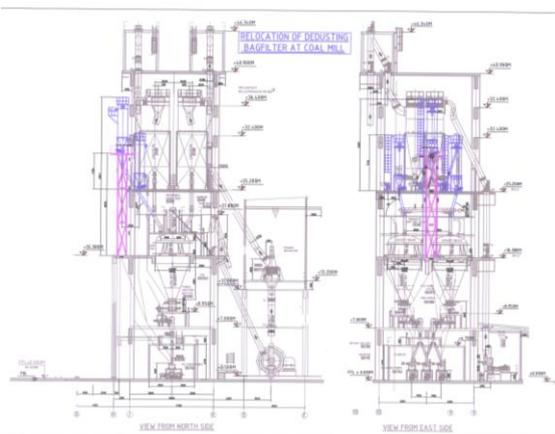
Fig.4 Bag filter position design after relocation
