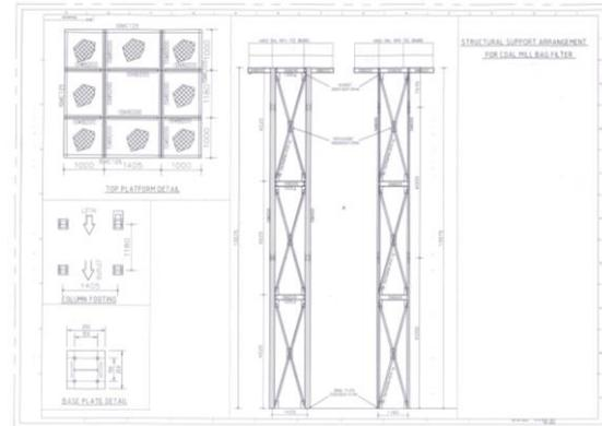
Fig.5 Structural support arrangement for bag filter
