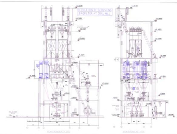
Fig.3 Bag filter position design before relocation
