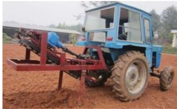
Fig. 3 Tapioca harvester Attached with tractor
