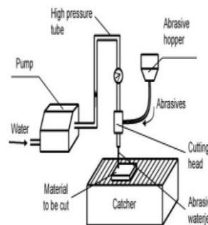
Fig. 1 Outline of abrasive water jet machining
