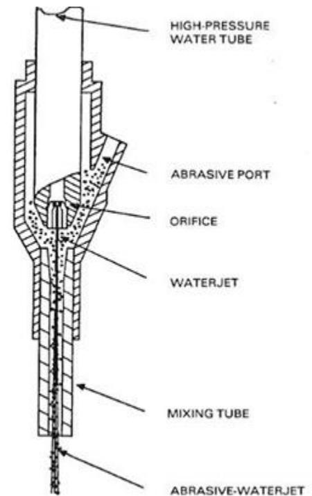
Fig.2 Abrasive nozzle
