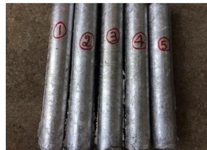
**Fig.2** Castings Produced by Stir Casting Process
