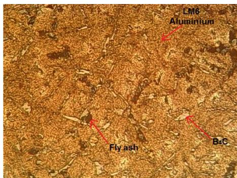
**Fig.3**Microstructure of LM6 – B<sub>4</sub>C – Fly ash reinforced composites
