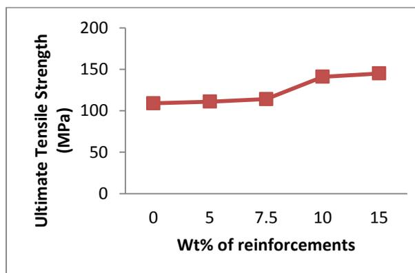
Fig.6 Variation of tensile strength with wt% of reinforcements
