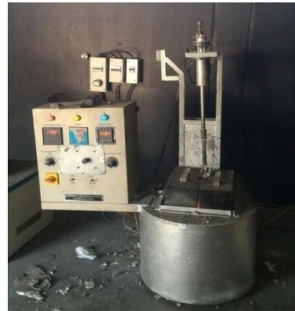
**Fig.1** Stir Casting Setup
