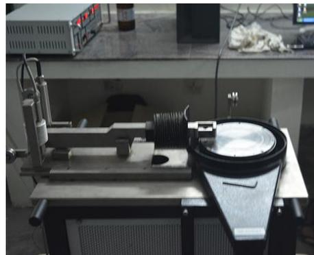
Fig.7. Pin – on – disc apparatus
