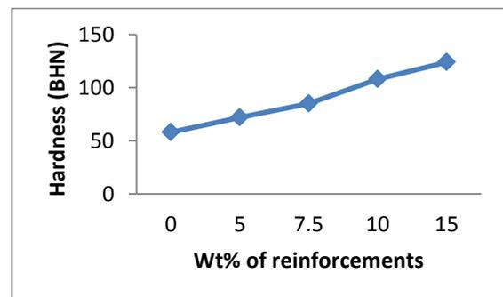
**Fig.5** Variation of hardness with wt% of reinforcements
