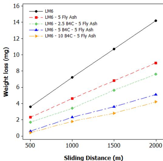
Fig.9 Variation of weight loss against sliding distance
