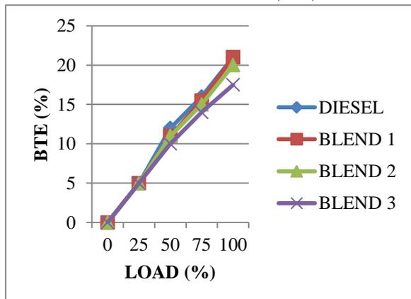
Fig.3: Engine load vs Brake Thermal Efficiency
