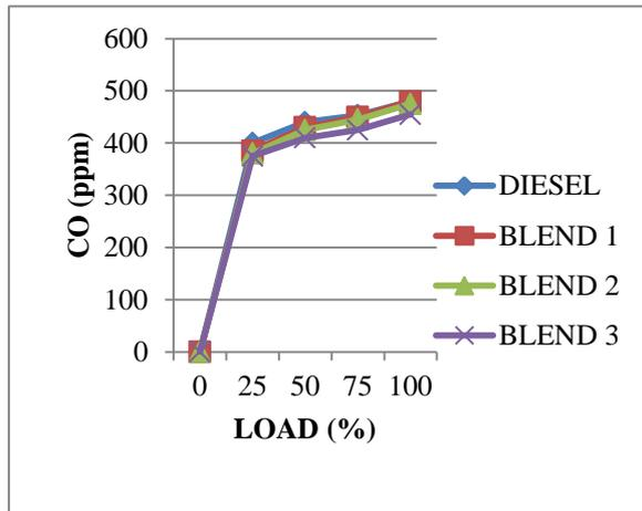
Fig.5: Engine load vs Carbon Monoxide
