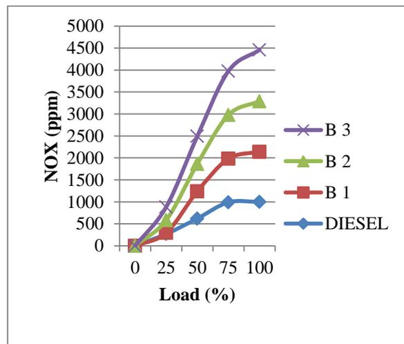
Fig.7: Engine load vs NOx
