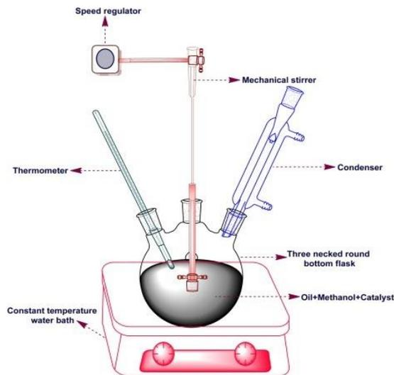
Fig.1: Transesterification setup
