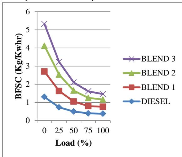
Fig.2: Engine load vs Brake specific fuel consumption
