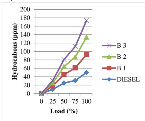
Fig.6: Engine load vs Hydrocarbons
