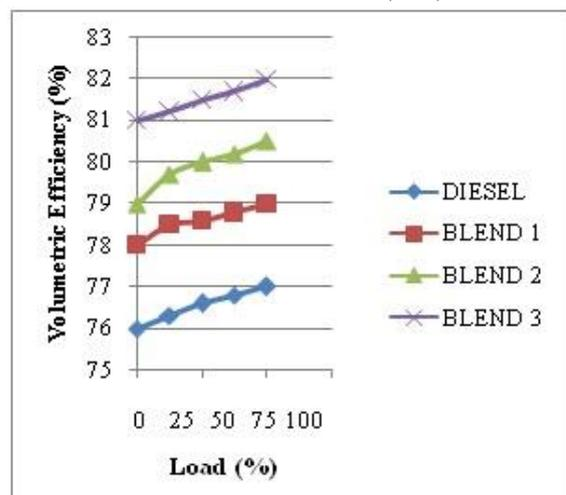
Fig.4: Engine load vs Volumetric Efficiency
