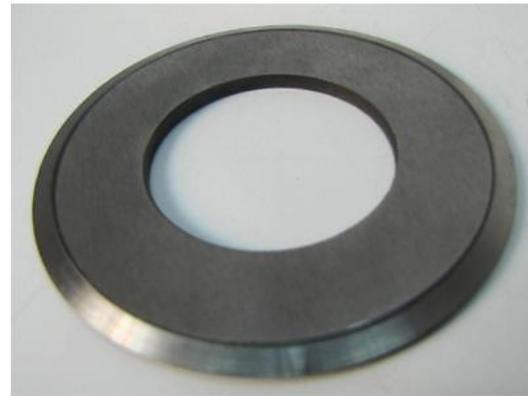
Fig. 3 Rotary Blade
