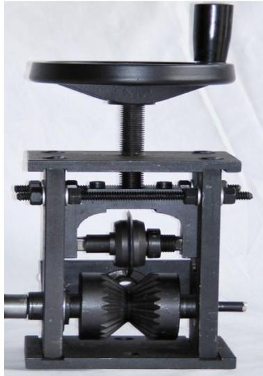
Fig. 1 Copper wire stripper machine
