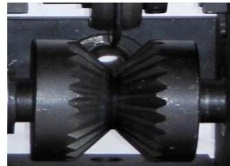
Fig. 1 V-Groove grip and blade setting
