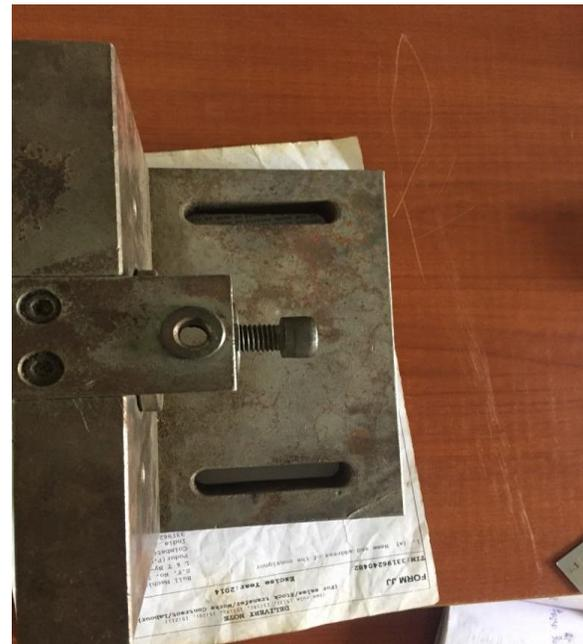
To overcome from this problem which is raised we have fixed an extra shaft in the other side. By help of that shaft we can able to rotate the shaft by 90 Degree.
