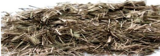
Fig. 3 Basalt fiber
