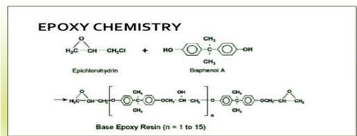
Fig.2 Chemical structure of epoxy resin
