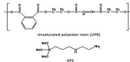
Fig.3 Chemical structure of polyester resin
