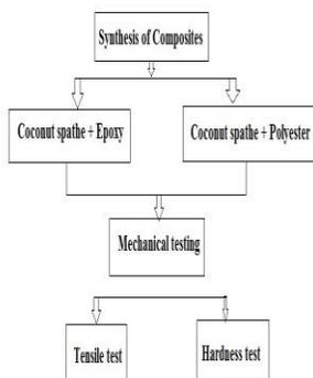
Fig.5 Synthesis of Coconut spathe fiber reinforced composites
