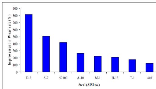
Fig .1 Improvement in Wear Rate due to Deep Cryogenic
