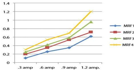
Figure 5. Brake torque "x" vs. Current (at 1000 rpm).
