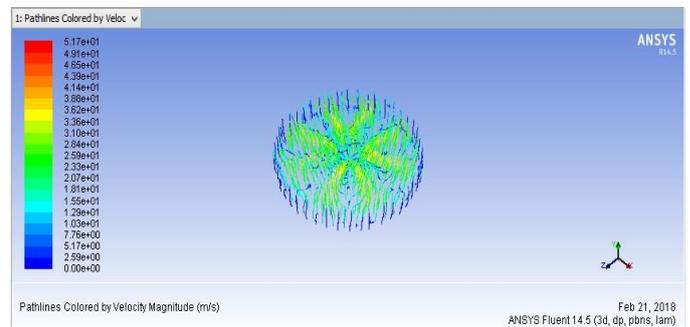
Fig .10 Pathlines coloured by velocity magnitude (m/s)
