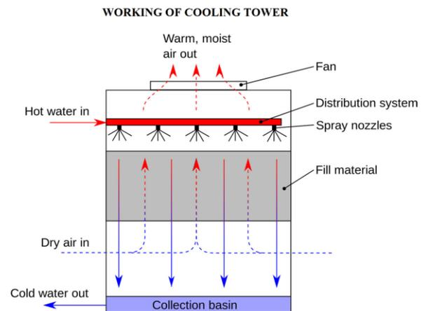
Fig .1 Working of Cooling Tower
