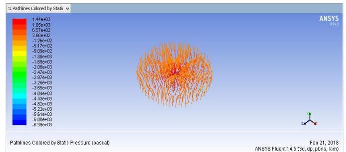
Fig .11 Pathlines coloured by static pressure (pascal)
