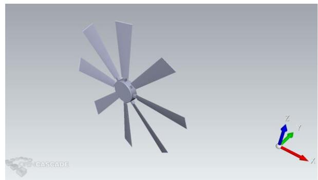
Fig .3 Modelling of cooling tower fan
