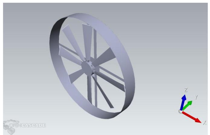
Fig .4 Modelling of cooling tower fan with outer casing
