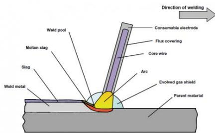
Fig.3 ARC Welding Process
