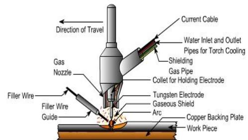
Fig.1 TIG Welding Process
