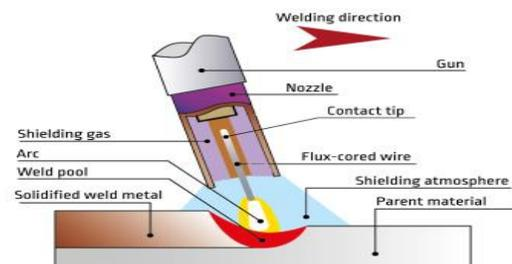
Fig.2 MIG Welding Process
