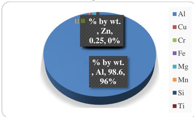
Fig.6 Al 6061-6063 alloy Composition material
