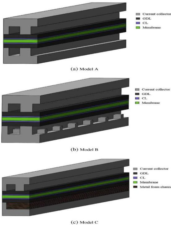
Fig. 9 Two parallel flow channels, (b) Locally baffle restricted flow channels and (c) Metal foam as a flow distributor. [1]
