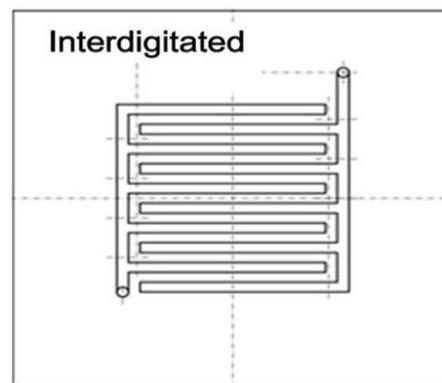
Fig. 8 Interdigitated flow field.[13]
