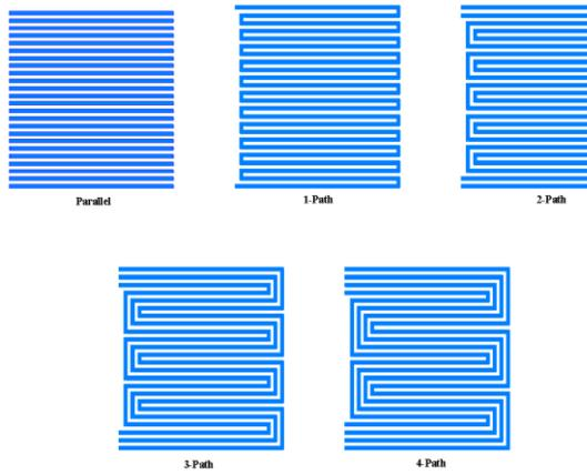
Fig. 2 Different flow field patterns [12]
