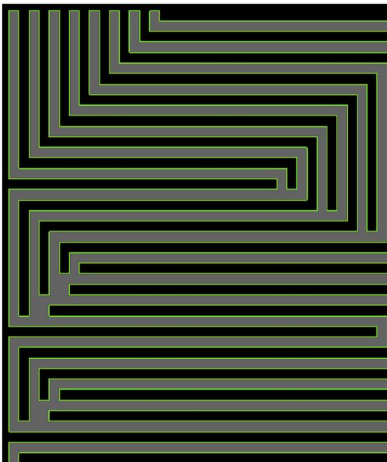
Fig. 3 Cascade type serpentine flow field [2]
