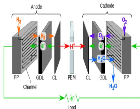
Fig. 1 Arrangement of PEM fuel cell
