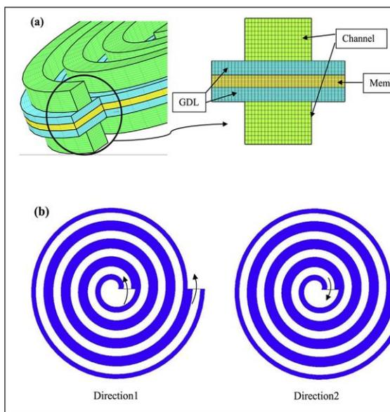
Fig. 10(a) Three-dimensional computational domain, (b) gas flow directions. [11]
