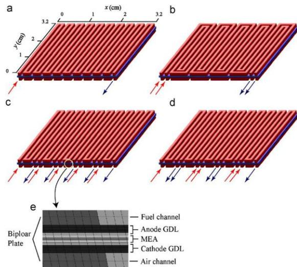
Fig. 4(a) single channel flow-field; (b) double channel flow-field; (c) cyclic-singlechannel flow-field; (d) symmetric-single channel flow-field; (e) the detailed schematic of computational domain.[3]
