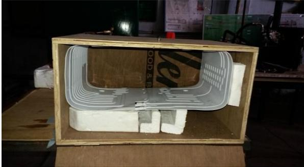
Fig-4: Evaporator used in experiment
