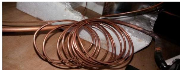
Fig-3: Throttling device used in experiment
