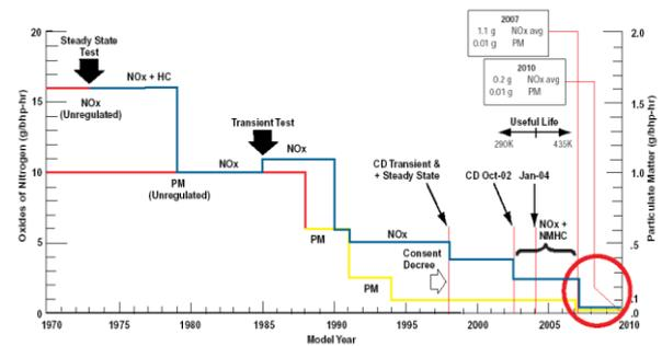
Fig.3. EPA Heavy Duty Engine Emission Standards
