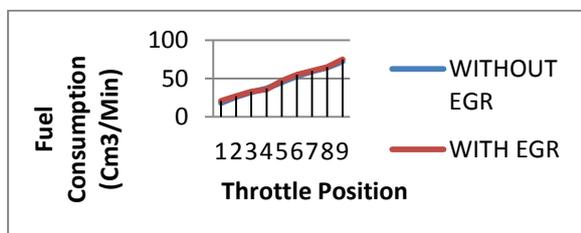
Figure 2. The effect of EGR on fuel consumption
