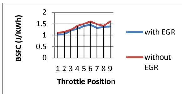
Figure3. Effect of EGR on the brake specific fuel consumption
