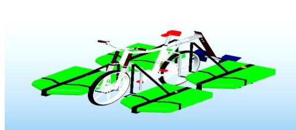
Fig. 2 3D view of amphibious cycle
