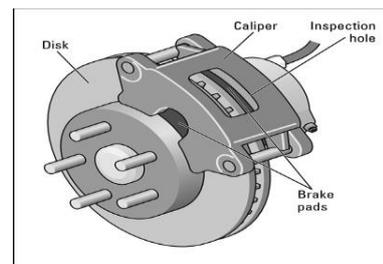
Fig.2 Disc Brake
