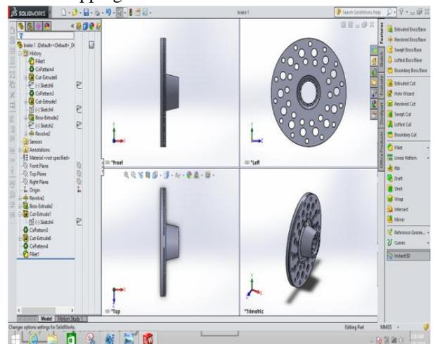
Fig 5.solid works diagram of disc brake
