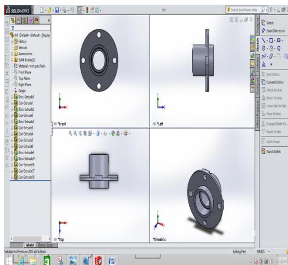
Fig 6. solid work diagram of wheel hub
