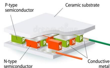
Fig. 3 Thermo electric material
