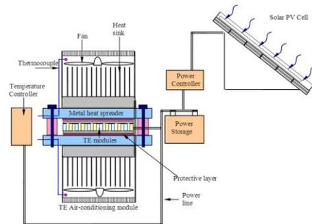
Fig. 4 Solar refrigeration with dissimilar metal
