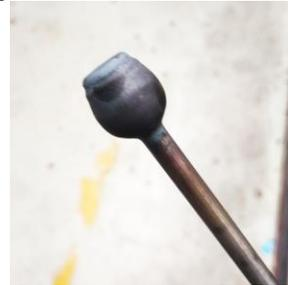
Figure 4. Unforged bar bulb
