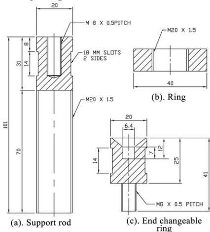
Figure 11. Upsetter bar guide bush – Modified design
