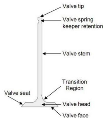
Figure 1. Parts of engine valve
