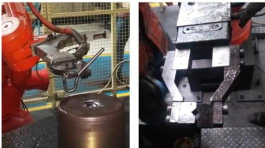
Figure 8. Gripper misalignment
