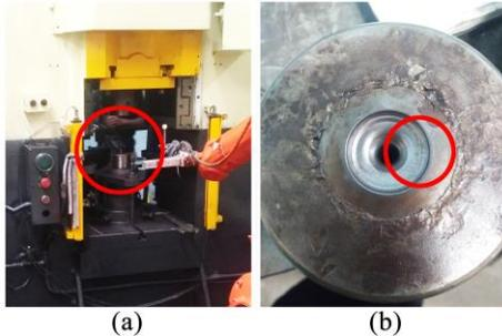
Figure 7. (a). Job stuck at die (b). Die damage
