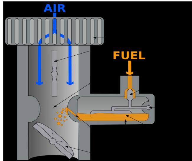
Fig. 5 Carburetor working
