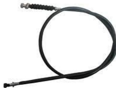
Fig. 3 Accelerate wire
