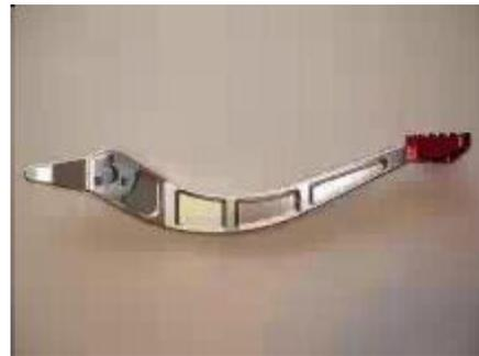
Fig. 2 Accelerator lever
