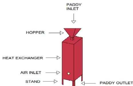
Fig. 3 3-Dimensional view of heat exchanger
