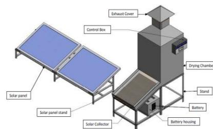
Fig. 5 Experimental setup
